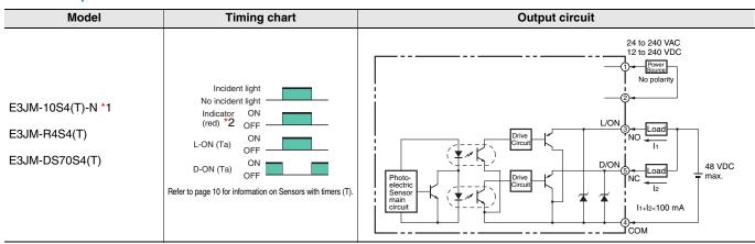
Note: Connect terminal 1 to any polarity and terminal 2 to the power supply because there is no polarity on the Emitter side.
